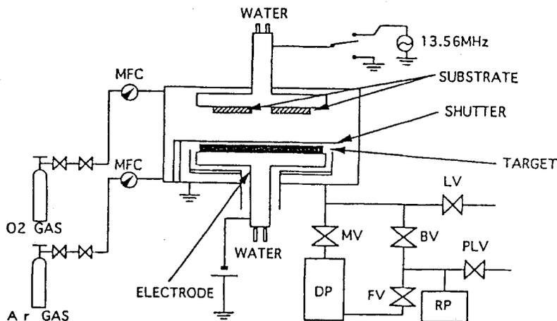
FIGURE 2 Schematic of sputtering apparatus used to deposit copper (Cu) on polyimide (PI) substrates.
