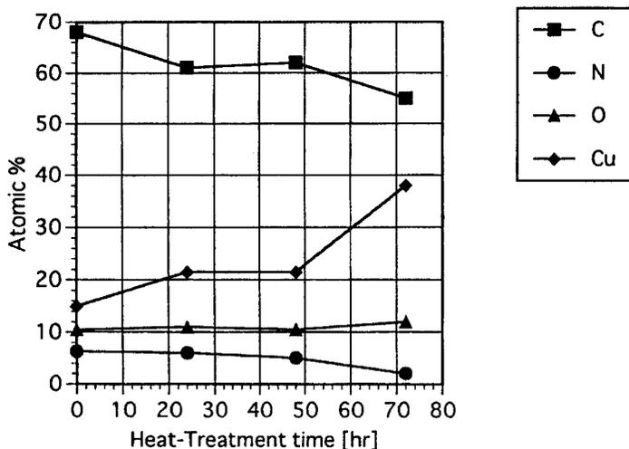
FIGURE 5 AES analysis of carbon (C), nitrogen (N), oxygen (O), and copper (Cu) on the peeled Cu surface of a Cu/PMDA-ODA laminate.
