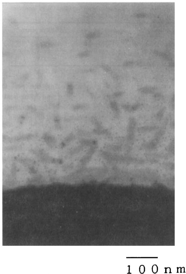
FIGURE 3 TEM micrograph of the interface of a Cu/PMDA-ODA laminate after heat treatment at 150°C in air.
