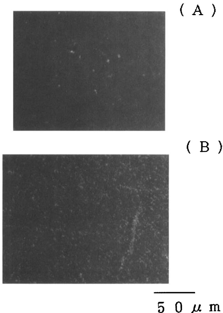
FIGURE 7 Optical micrograph of a peeled PI surface of a Cu/BPDA-ODA laminate: (A) before heat treatment and (B) after heat treatment at 150°C in air for 24 hr.
