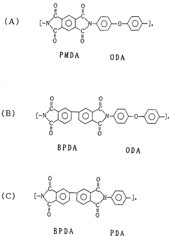
FIGURE 1 Structural formulas of the polyimides used as substrates in copper/polyimide laminates. (A) Kapton-V (PMDA-ODA), (B) Upilex-R (BPDA-ODA), and (C) Upilex-S (BPDA-PDA).
