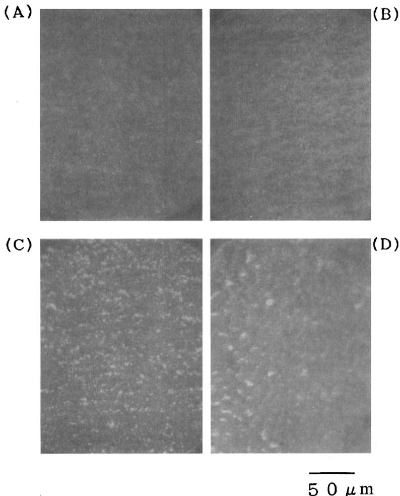
FIGURE 4 Optical micrograph of a peeled PI surface in a Cu/PMDA-ODA laminate: (A) before heat treatment, (B) after heat treatment at 150°C in air for 24 hr, (C) for 48 hr, and (D) for 72 hr.
