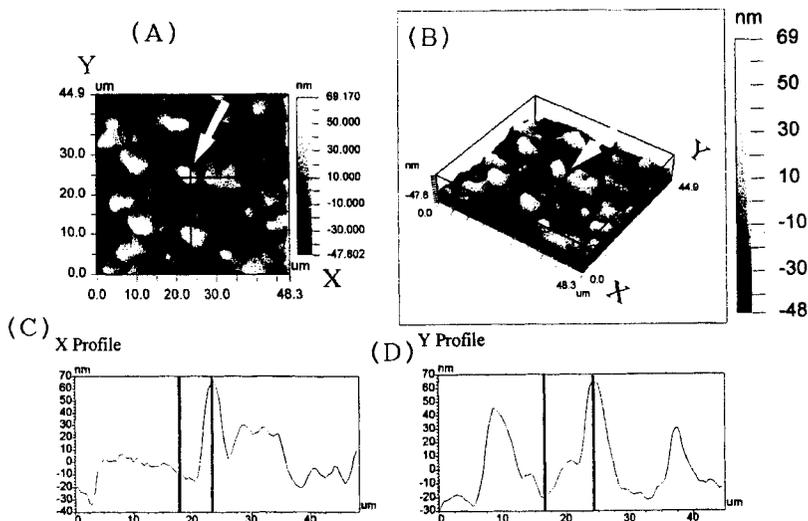
FIGURE 9 The topographies of the Cu bright spots on the peeled PI surface treated at 150°C in air for 3 days. (A) and (B) show 2-D and 3-D topographies of these surfaces. (C) and (D) show the sectional plans for X-axis and Y-axis, respectively.
